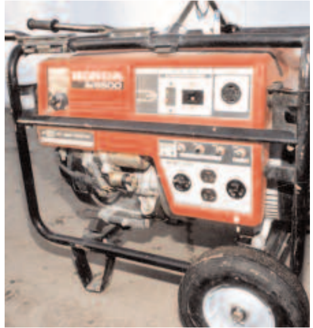
Even small, portable generators such as this can easily produce 1 percent of their exhaust as carbon monoxide.
